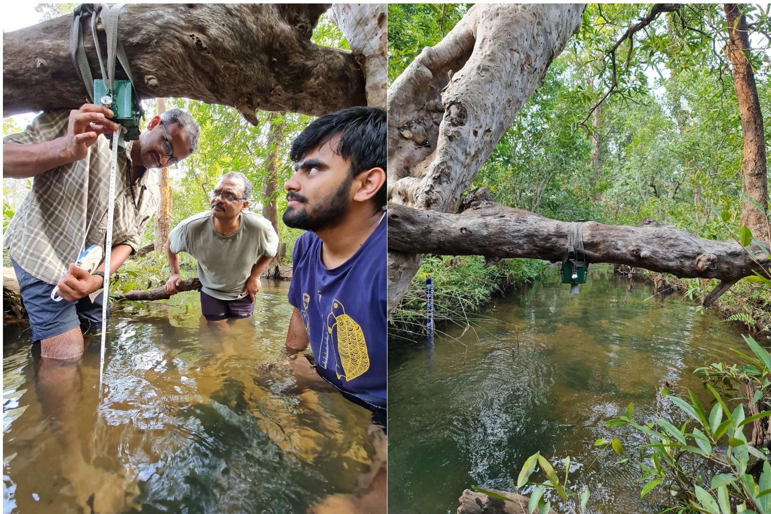
FIGURE 18: FIELD INSTALLATION OF AN ACOUSTIC WATER LEVEL RECORDER (WLR)
