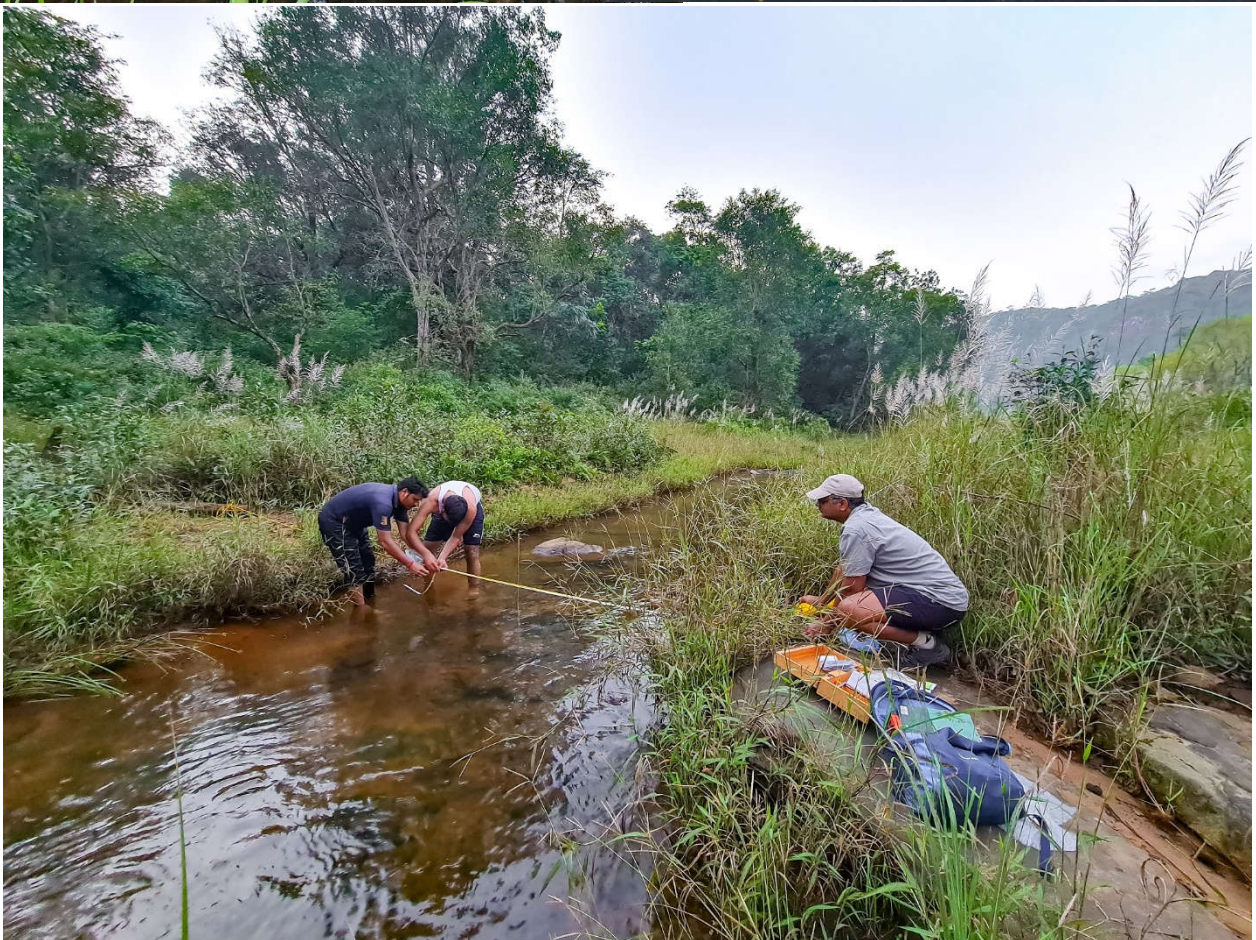
FIGURE 21 MEASUREMENTS OF STREAM WIDTH, DEPTH AND FLOW VELOCITY. FOREST PATROLLING STAFF OCCASIONALLY PARTICIPATED DURING THESE SURVEYS
